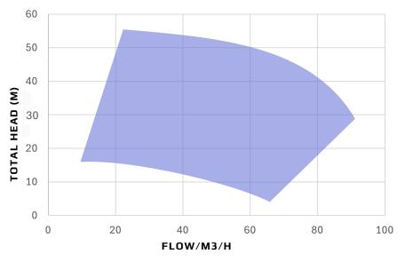
\*Pump performance curve is based on water with a SG=1.0 and without additional accessories.
